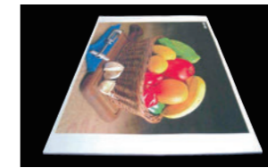
Oil-based ink causes minimal paper deformation
