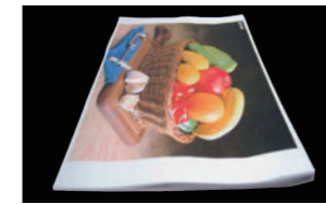
Water-based ink results in deformation such as swelling and waviness
