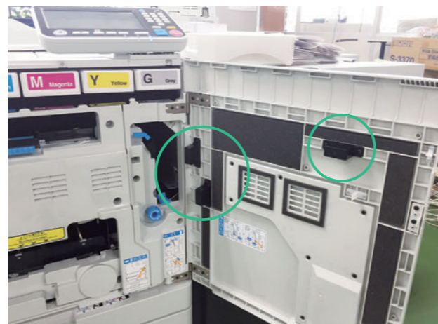
An example of a recycled plastic part used in the ComColor GD series
