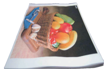
Water-based inks tend to cause waves, curls, and other deformities.
