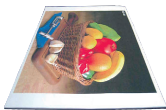
Oil-based inks reduce such deformities.
